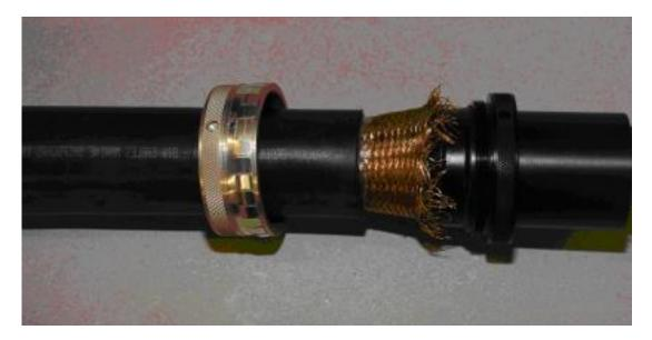
IMPORTANT: Engage the threads on the silver ring and the black ring and turn only the knurled ring on the black part to tighten. Be careful to not twist the cable braid.
