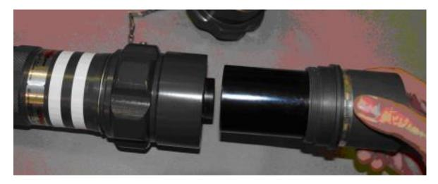
When the front plug shell is firmly screwed into position, install the front retaining washer and snap ring on the contact using the supplied tools.
